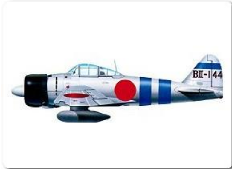
Mitsubishi A6M3 Zero Carrier Fighter Max. Weight: 5,828lbs / Max. Speed: 336 mph
