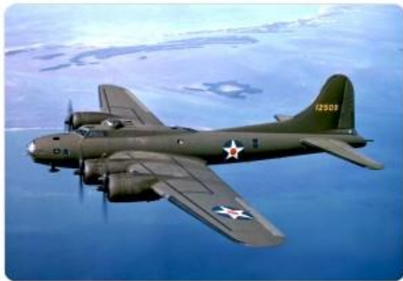
Boeing B-17E Flying Fortress Heavy Bomber Max. Weight: 51,000lbs / Max. Speed: 318 mph
