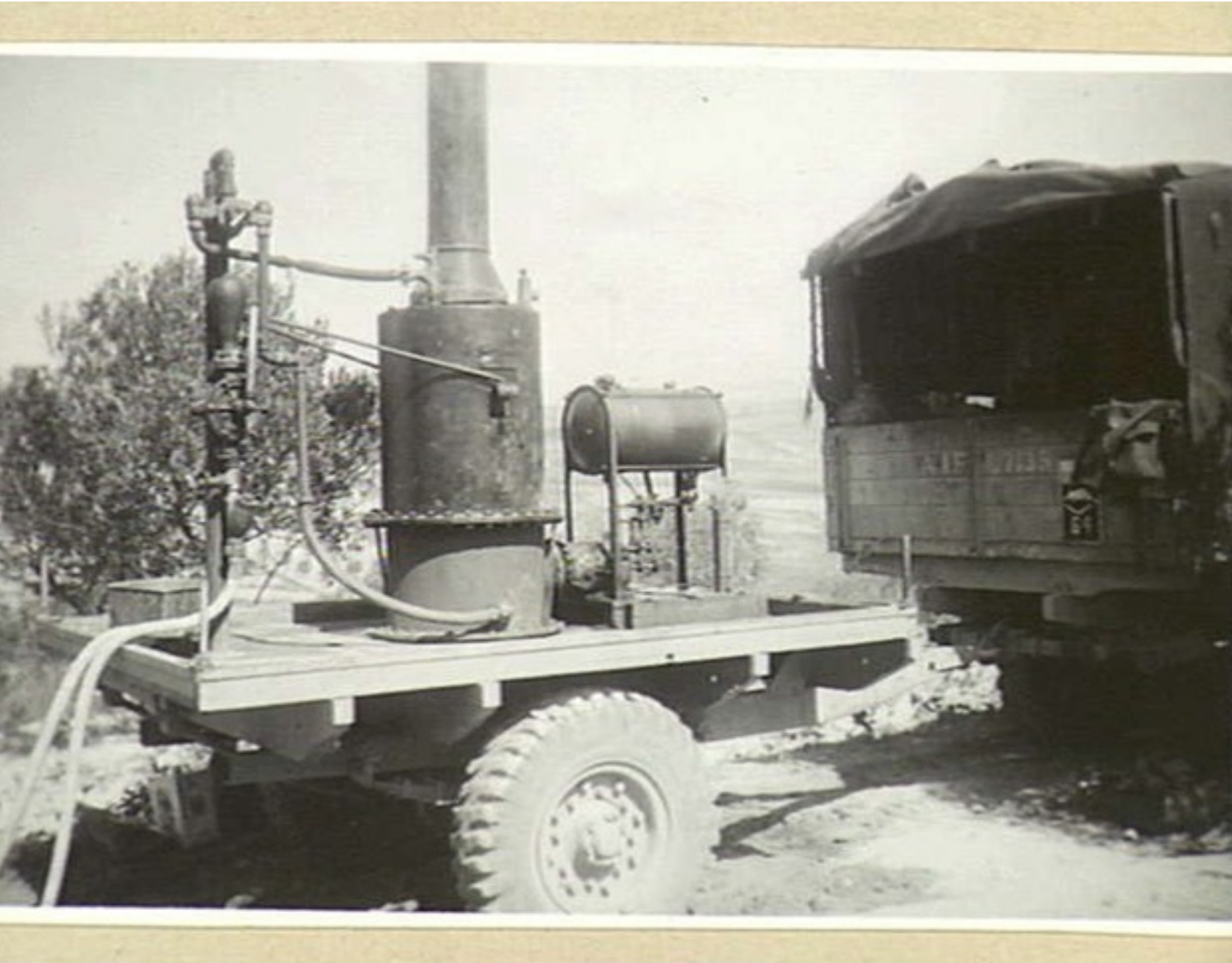
LATTAQUIE, SYRIA, 1942-04-02. THE BOILER TRUCK WITH THIMBLE BOILER AND RUTHERFORD BURNER, OF THE 9TH AUSTRALIAN DIVISION MOBILE BATH UNIT, IN OPERATION.
